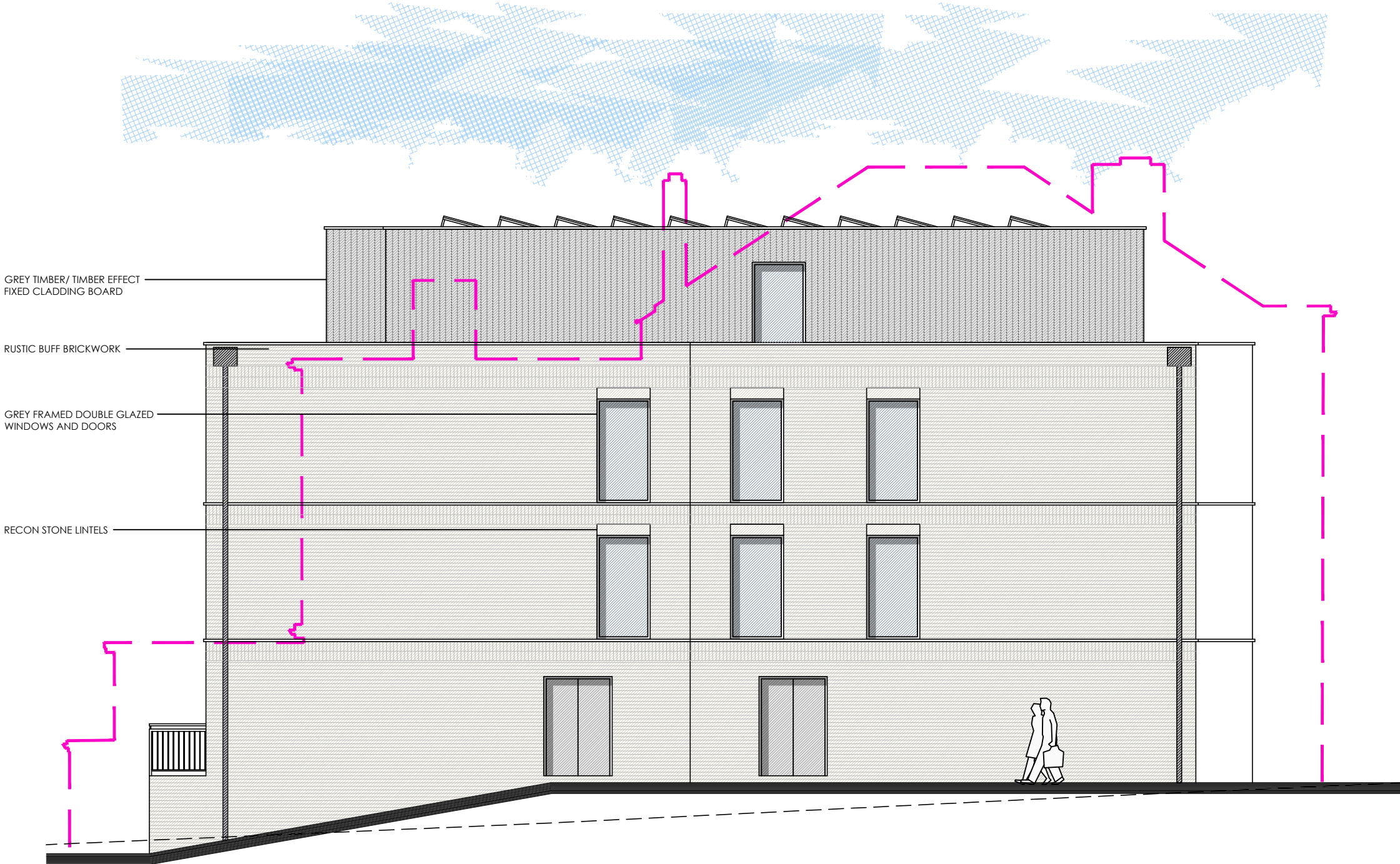
PROPOSED WEST ELEVATION SCALE 1:100
